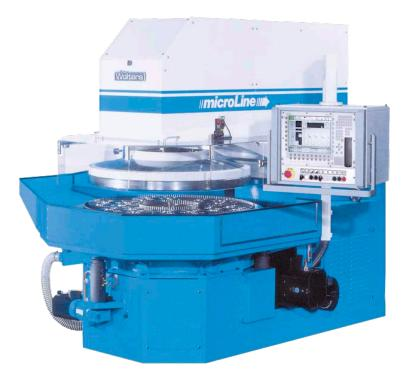
PETER WOLTERS AC 1200 double-side batch processing machine has been designed for high-precision series processing work pieces. Due to its modular construction, AC 1200 can be used as a fine grinding, lapping, honing, and polishing machine.
