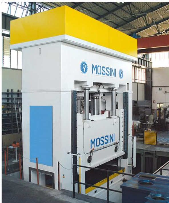
PO-2M-T-2000 (TRIPLE ACTION PRESS; TABLE SIZE 4500x2500 mm.)
