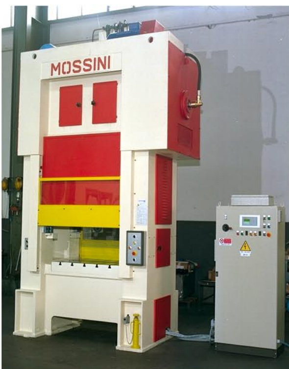
PDM-2B-V-100 (HIGH SPEED PRESS; TABLE SIZE 1250x900 mm.)
