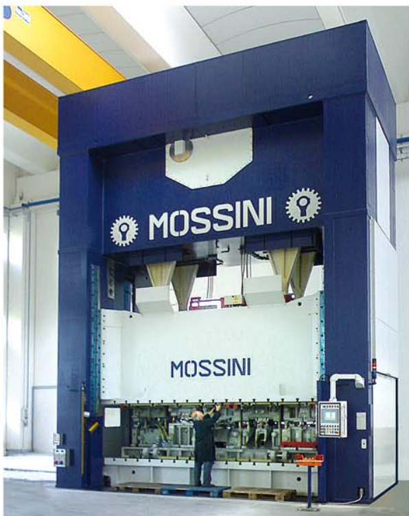
PDM-4B-1000 (ECCENTRIC PRESS; TABLE SIZE 5000x2500 mm.)
