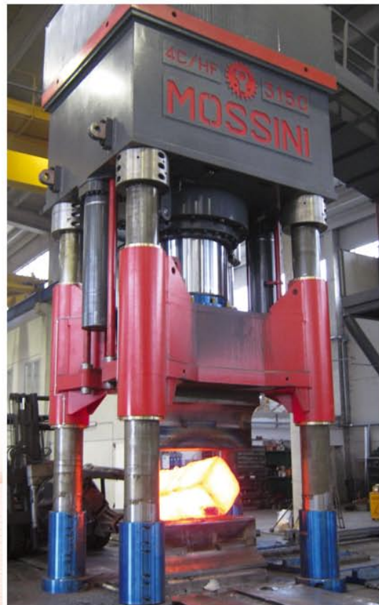
HOT FORGING PRESSES
