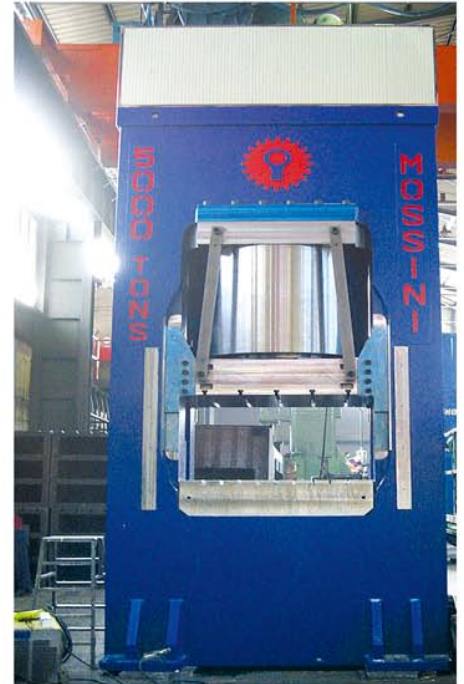
PLATE HEAT EXCHANGER PRESSES
