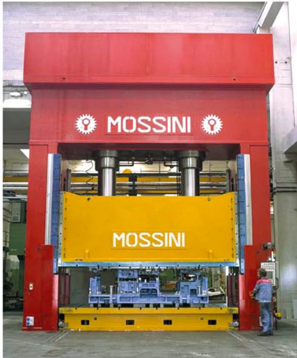
PO-2M-P-2000 (TRY-OUT PRESS; TABLE SIZE 5000x2500 mm.)
