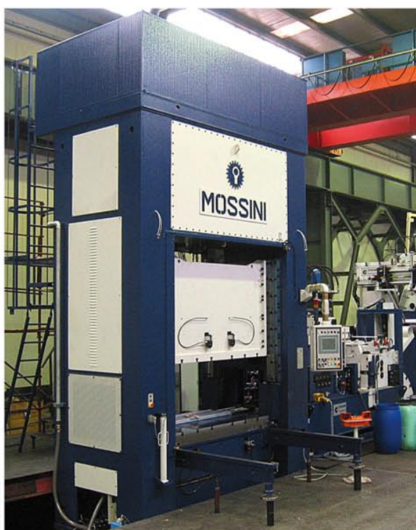
PDM-2B-500 (AUTOMATIC STROKE CHANGE; TABLE SIZE 2200x1250 mm.)
