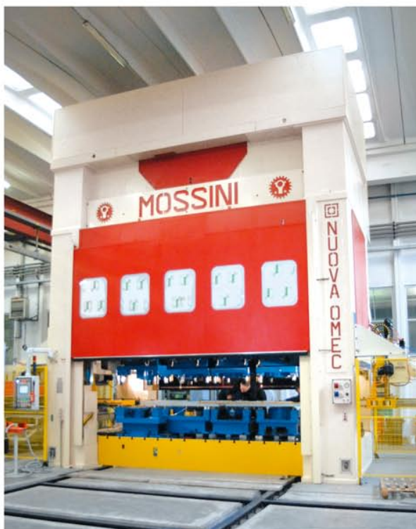
PDM-4B-LD-1250 (LINK DRIVE PRESS; TABLE SIZE 4500x2200 mm.)
