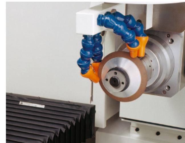
Automatic changing of the grinding wheels via HSK spindle adapters
