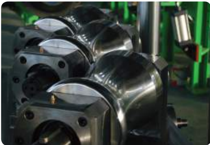
Detail Rohrriechmaschine Detail Tube Straightener
